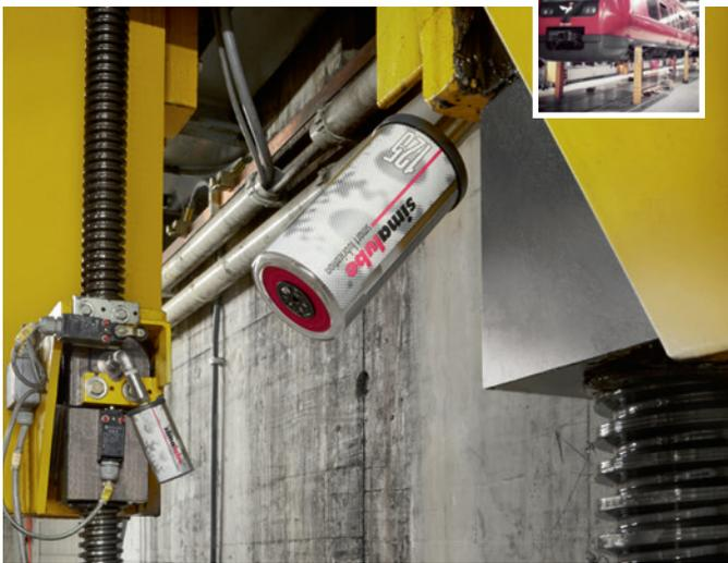
The spindles of a lifting station for railway wagons and locomotives are lubricated with 125 ml simalube over 12 months.
