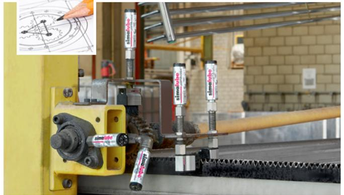
15 ml simalube lubricators with brushes constantly supply the rack of a loading machine with oil. Additional 15 ml simalube lubricators lubricate the flange bearings with grease.
