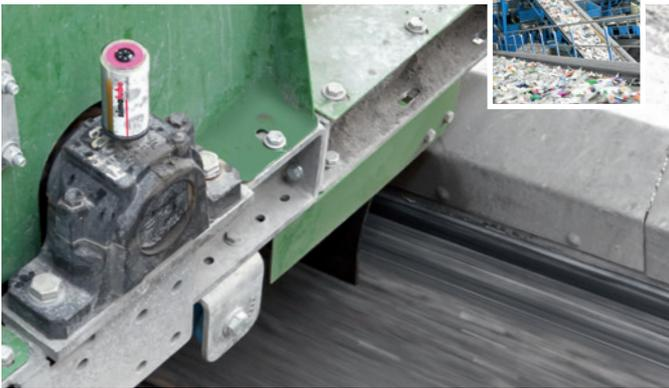
A 125 ml simalube lubricates the pedestal bearing of a conveyor belt.
