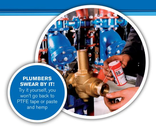
Loctite 55 is the must have product for sealing pipe threads and fittings. It allows parts to be backed off for adjustment which is why it has become one of the most popular pipe sealing products. Applied simply by wrapping the sealing cord around the thread, as described on the pack, which produces a pressure tight joint that can be realigned without the need for reapplication of the cord.
