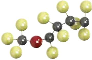
Perfluoroelastomers (FFKM) have a fully fluorinated polymer backbone resulting in a fluorine content >71%. As the material is free from carbon-hydrogen bonds in the polymer chain, the FFKM materials offer the ultimate thermo-chemical resistance.
