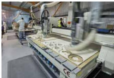
The **CNC machining work cell** is equipped with 3 axis machining centres, or routers, to profile cut three dimensional insulation board for the appliance sector.
