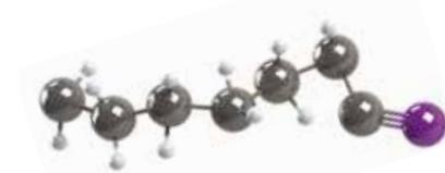
Hydrogenated nitrile rubber (HNBR) is a highly saturated copolymer of acrylonitrile (ACN) and butadiene.
