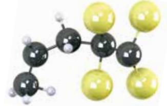
The most common forms of FEPM are categorized within ASTM D 1418-01. These grades are alternating copolymers of tetrafluoroethylene and propylene, with a fluorine content of ~54%. Such chemical structures offer excellent heat resistance, exceptional chemical resistance (significantly to alkalis and amines), along with high electrical resistivity.
