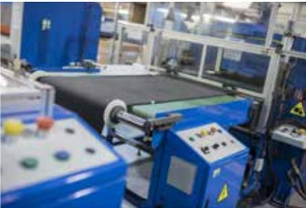
Our range of high speed, **precision die-cutting press** technology can support serial OEM schedule orders to cut seals and gaskets that offer both high quality and excellent manufacturing efficiencies to our clients. We have recently added additional capability to supply large dimension kiss-cut parts that offer you an improved assembly process.
