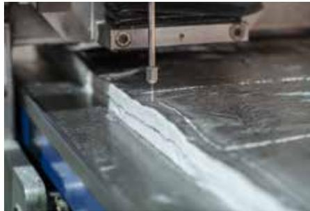
Our **water-jet work cell** is capable of precision profile cutting a wide range of materials from insulation blanket or boards, cellular foam to metals. This CNC driven equipment is ideal for quick response to individual orders or mid-high volume manufacture.
