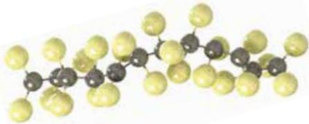
PTFE (polytetrafluoroethylene) is a synthetic, thermoplastic polymer which offers exceptional chemical resistance over a wide range of temperatures and offers extremely low levels of friction.
