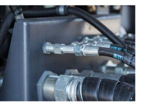
Rather than simply replacing like-for-like, ERIKS' technicians used the opportunity to upgrade components where improved hose technologies were available. New hoses with better flow and pressure ratings were specified and installed, enhancing the simulator's hydraulic performance.
