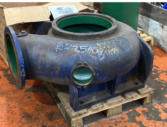
Dirty water return pump before undergoing overhaul
