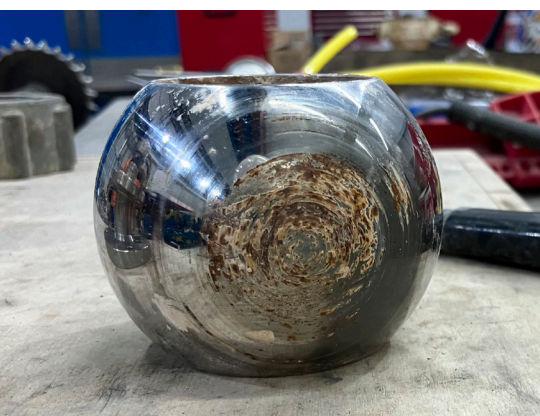
Worn ball from the ceramic seated valves
