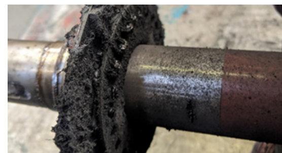
Deteriorated and contaminated Drive End
