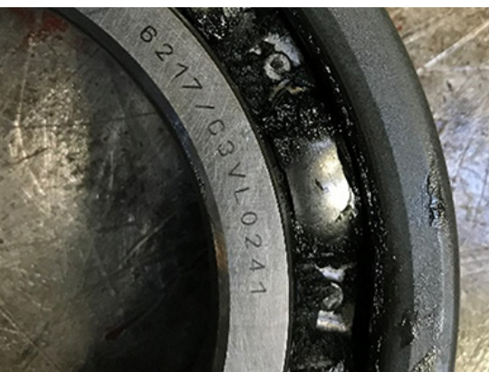
Bearing displaying signs of contaminated lubricant
