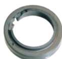
The cracked outer sealing lip of this wiper seal shows damage caused by heat
