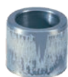
Particle contamination has scored the surface of this cushion bush, resulting in a loss of cushioning effect
