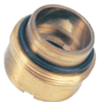
Gland and seal showing wear resulting from excessive side loading. Brass 'paste' on seal is a mixture of gland material and hydraulic fluid
