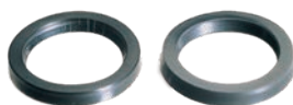
Contamination damage is apparent in this rod seal, where the serrations are worn completely away. The seal on the right is new, shown for comparison.
