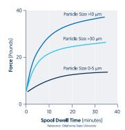
Valve silting / stiction from particle build-up between moving surfaces increases valve shifting force. The highest force is required when the valve is challenged by particles in the dynamic clearance size range (~10 µm)
