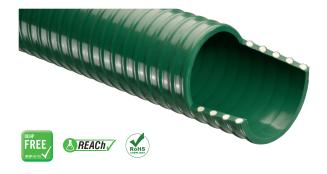
A standard medium duty PVC hose, reinforced with a semirigid crush resistant PVC helix. It is tough flexible and extremely durable under normal operating conditions. It has outstanding resistance to the effects of the weather. Minimum frictional loss is achieved by the smooth bore.
