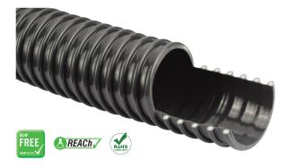
High flexibility lightweight PVC ducting hose, reinforced with a rigid crush resistant white PVC helix. It is tough, flexible and extremely durable under normal operating conditions. The cross section is maintained even when highly flexed. Minimum frictional loss is achieved by the smooth bore.
