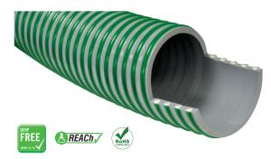
A medium weight PVC hose, manufactured from super elastic compounds to give increased flexibility. It is reinforced with a semi-rigid crush resistant PVC helix that is protected by a raised scuff strip. It is tough, flexible and extremely durable under normal operating conditions. It has outstanding resistance to the effects of weather. Minimum frictional loss is achieved by the smooth bore.
