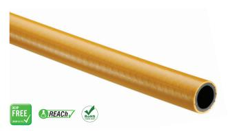
Manufactured from abrasion resistant PVC, offering excellent flexibility and kink resistance, this hose is a highly versatile reinforced PVC hose capable of working at 20 Bar.
