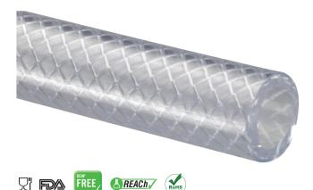
A lightweight PVC hose, reinforced with high tensile polyester fibers. The clear braided PVC hose is tough, flexible and extremely durable under normal operating conditions. Manufactured from FDA approved ingredients. The braided PVC hose is suitable for food contact applications and is resistant to a wide range of chemicals. Minimum frictional loss is achieved by the smooth bore.
