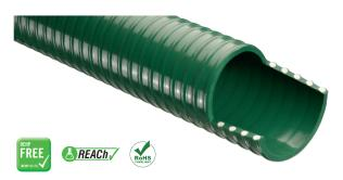
A premium medium weight PVC hose, reinforced with a semirigid crush resistant PVC helix. It is tough, flexible and extremely durable under normal operating conditions. It has outstanding resistance to the effects of weather. Minimum frictional loss is achieved by the smooth bore.
