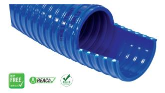
A light weight oil resistant PVC hose, reinforced with a semirigid crush resistant PVC helix. It is tough, flexible and extremely durable under normal operating conditions. Manufactured from a compound containing nitrile, this hose is designed for the transportation of fuel oils. Minimum frictional loss is achieved by the smooth bore.
