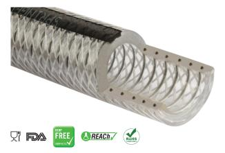
Springflex<sup>™</sup> braided food quality hose is manufactured from two layers of soft PVC compound. It is constructed with a steel spiral embedded in the first layer and a polyester yarn reinforcement between the first and second layer. This heavy duty hose is extremely tough and flexible and designed for the suction and delivery of liquid foodstuffs in arduous applications.
