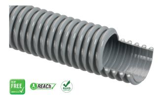
A medium weight PVC ducting hose, reinforced with a semirigid crush resistant white PVC helix. It is tough, flexible and extremely durable under normal operating conditions. The cross section is maintained even when highly flexed. Minimum frictional loss is achieved by the smooth bore.
